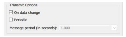
When event-based transmission is enabled, messages are transmitted only at those time steps when a change in message data is detected. When the input data matches the most recent transmission for a given message ID, the message is not re-transmitted.
